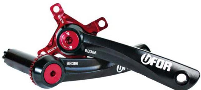
*It could also be used on threaded BB shells, thanks to the threaded reducer cups for 30mm spindles. Moreover, it will also offer greatly improved performance compared to 24mm integrated systems.*
